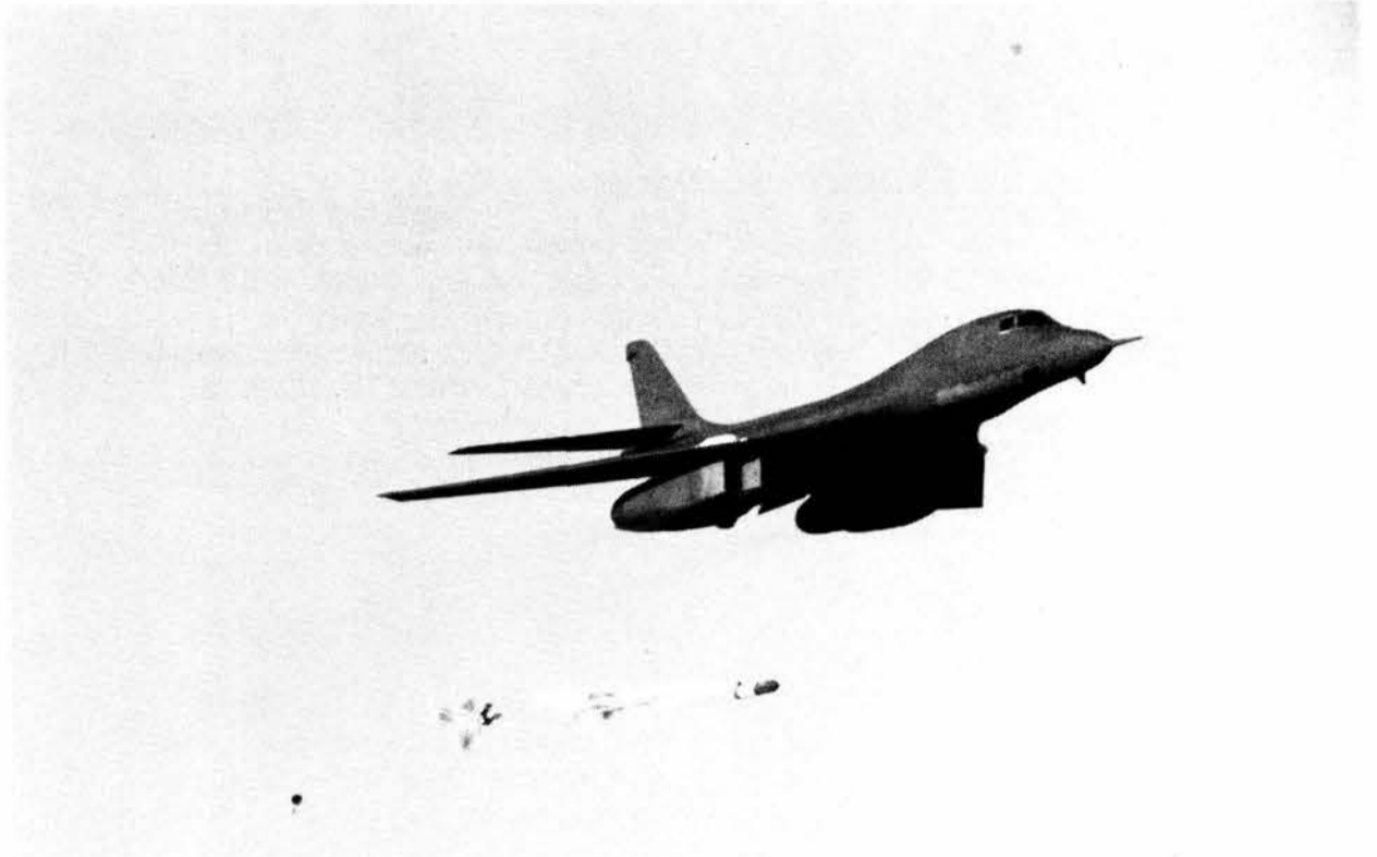
B-1 bomber drops a parachute retarded B83 weapon shape at about Mach 1 during a test series earlier this summer at Tonopah Test Range. See article starting on page five.
